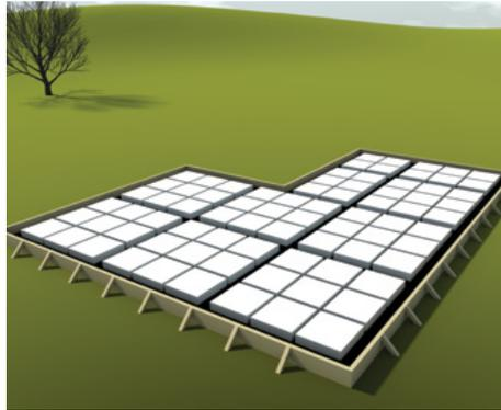
**5** Directly on top of this polythene membrane, we now construct a RibRaft® floor to a height of 320mm\*. [\*Sizes may change depending on the specific solution designed for your site.]
