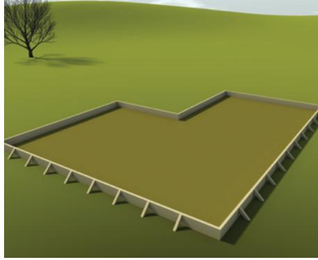
**2** The floorslab area is boxed to specification, but you will notice the height of the boxing is higher than a standard RibRaft®.
