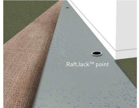
**1** A small team of qualified tradesmen will enter the house and from the building's floor plans identify and uncover the RaftJack™ points within the concrete floor. The RaftJack™ points are positioned clear of wall framing for ease of access. As a result, no structural element of the house will be disturbed. Internal walls and cladding remain intact throughout. Only floor coverings require removal for access.
