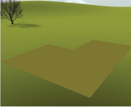
**1** As with Firth's standard RibRaft® floors, organic topsoil is removed on the building site.
