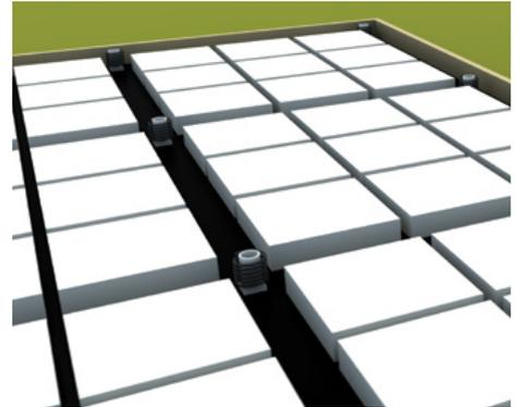
**6** In specified points within the RibRaft™ slab construction (clear of any wall framing), predetermined by engineers, a new innovative RaftJack™ housing is installed within the top slab.
