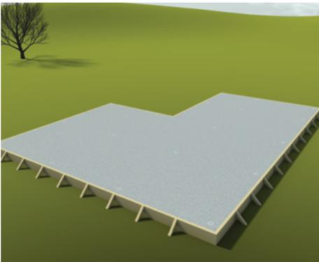
**7** The specifically engineered seismic resilient Firth concrete mix coupled with high ductility reinforcement (designed to MBIE guidelines) is poured within an engineered grid of polystyrene and reinforcing rods and mesh.
