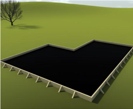
**4** After this first slab has been completed to the specified finish, and the floor has cured, a polythene membrane is placed on top, covering the entire floor. This acts as a vapour barrier between the slabs.
