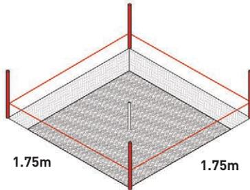
**MARK & DIG** To get started, mark out a 1750mm x 1750mm square base foundation on the site you want the fire pit located. The excavation is 100mm larger on each side of the completed planter.
