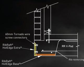
FIRTH RIBRAFT X-POD® BRICK VENEER HOTEDGE® & HOTEDGE BASE® FIRTH CONCRETE (MIX CODE IP2019X OR IP2519X)
