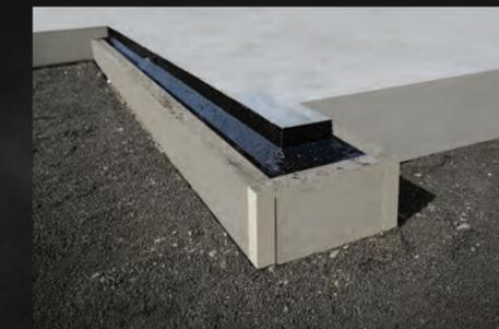
3 Boxing is removed, revealing a truly integrated, aesthetically finished thermal barrier to help achieve H1 compliance. Firth recommend two coats of acrylic paint should be applied to all exposed surfaces for optimum service life and insulation.
