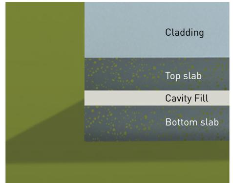
**4** A specially designed Firth concrete mix is pumped into the cavity to fill it and left to cure.
