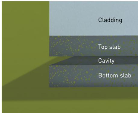
**3** Between the lower sunken slab and upper levelled slab there will clearly now be a cavity.
