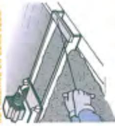
**11** FOR SMALL JOBS SLABS UP TO 100MM THICK A HAND TAMPER MAY BE USED
