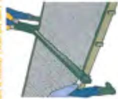
**12** POKER VIBRATORS SHOULD BE USED ALONG THE EDGES OF SLABS WHEN COMPACTING WITH A BEAM
