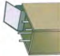
**8** FOR THIN SLABS USE A BEAM VIBRATOR. FOR COLUMNS, WALLS AND THICK SLABS USE POKER VIBRATORS
