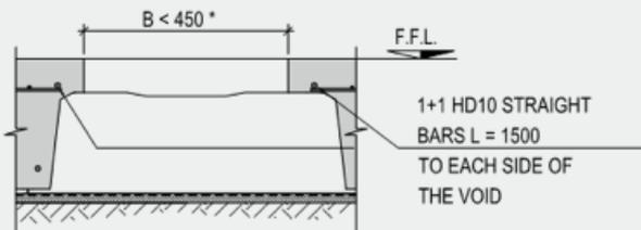
(\* IF B > 450 mm PLACE 2 HD10 CRACK CONTROL BARS @ 200 L = 2000 AT EACH CORNER OF THE PENETRATION
