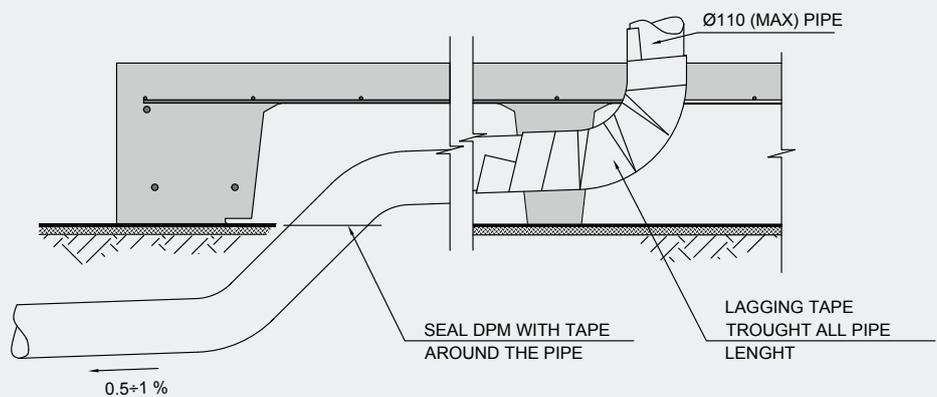
Use of Xpod® Mini Pods to create zone for pipes to run without compromising the ribs'
