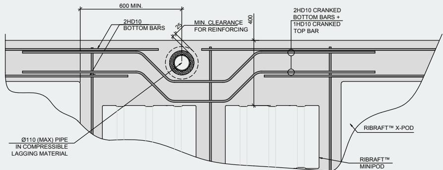
Use of Xpod® Mini Pods to create zone for pipes to penetrate slab.
