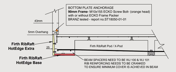
NZS3604 requires bolts securing bottom plates to have capacities greater than specified in clause 2.4.7. The ECKO M10 155mm screw bolt (orange top) has been BRANZ tested (ST18050-01-01) with 90mm framing and HotEdge Extra to demonstrate compliance. Alternative bolt arrangements can be used where cyclic testing demonstrates bolt capacities meet or exceed the requirements of NZS3604 or as required by the bracing system.
