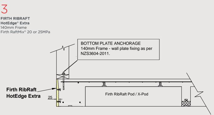
NOTE: This drawing can be used for the Construction Detail for 140mm framing with HotEdge Extra AND HotEdge Base.
