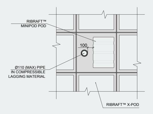
Typical drop down detail for sewer line to prevent it being visible at exterior of slab
