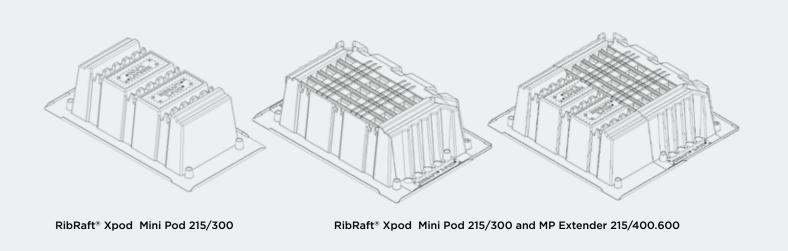
Firth RibRaft® X-Pod®s are placed directly on levelled ground and are arranged in such a way as to form a reinforced concrete floor slab with a grid of reinforced concrete ribs and edge beams when concrete is placed onto them. The RibRaft® Mini Pods Series X-Pod®s may be used to suit specific architecture layout and also to accommodate services.
