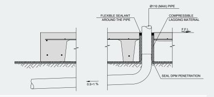
Details where large diameter pipe required through perimeter beam
