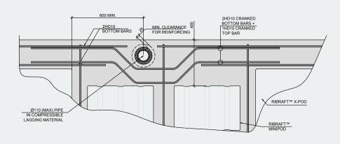
Use of Xpod® Mini Pods to create zone for pipes to penetrate slab.
